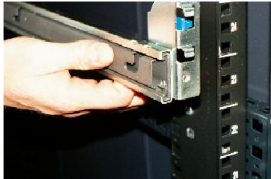
Figure 1 Numbered “U” Mounting Holes and Rapid Rail Installation
